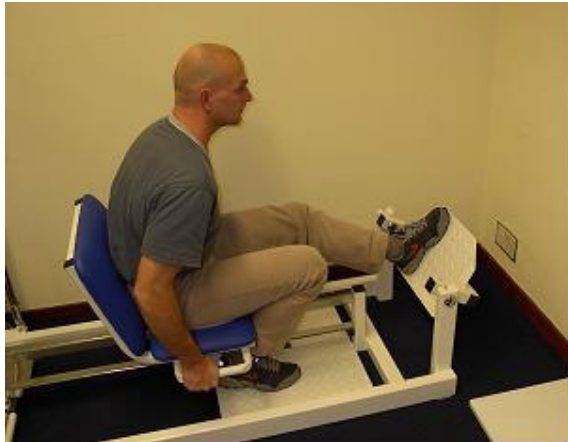
Figure 2 Testing maximal static force preferably in the smaller “skate angle”
